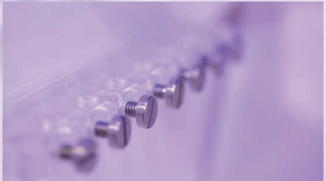
7 port probe holder array with titanium screws
